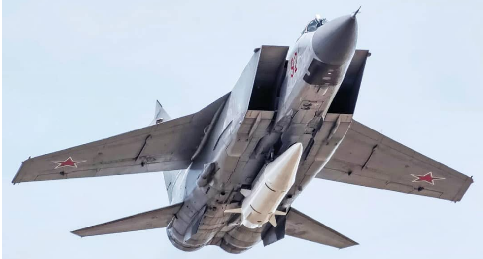
The Kh-47M2 Kinzhal operational hypersonic missile underneath a MiG-31K fighter jet.
